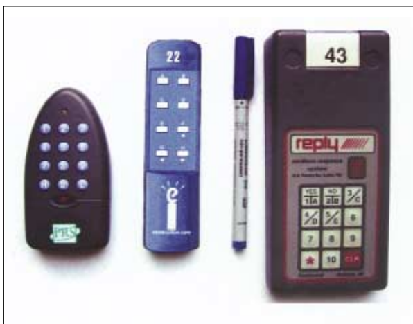
Fig. 1. Photograph of wireless keypads (from left), PRS keypad, CPS keypad, and Fleetwood keypad. The length of the pen is ~5.5 in/14 cm.
